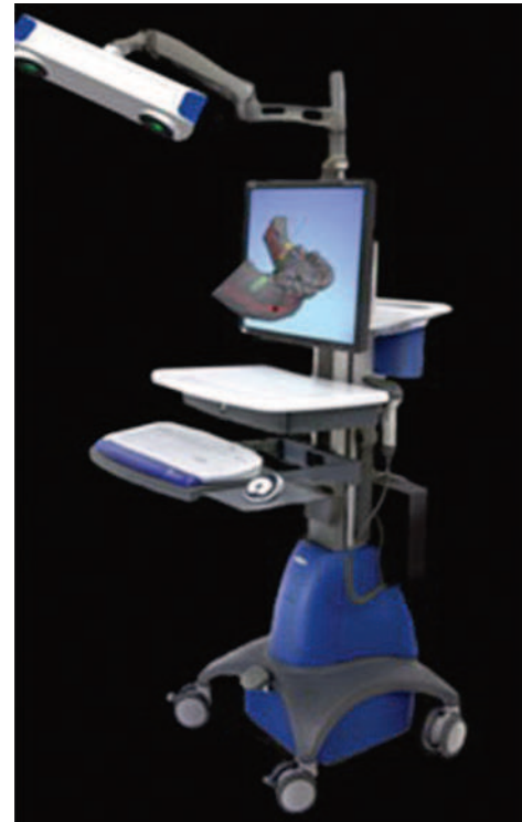
Fig. 84.5 Dental implant real-time navigation system with infrared stereovision cameras and a three-dimensional monitor display showing the reconstruction of a computed tomography-scanned mandible.
