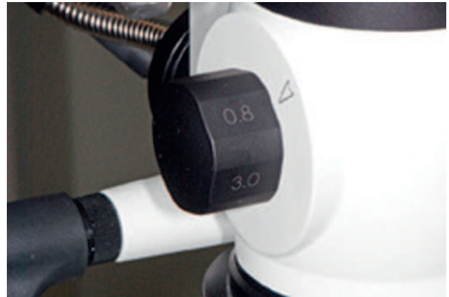
Fig. 67.26 Rotating magnification element with a field of view ranging from the full mouth to approximately 3 cm when using a 250-mm objective lens.
