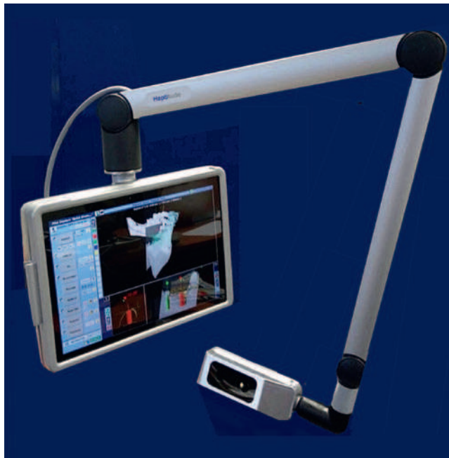
Fig. 84.1 Dental implant real-time navigation system (Open Pilot System, Stereovision Haptitude) with infrared stereovision cameras and a monitor display showing the three-dimensional ultrasonic reconstruction of a mandible with the planned implant position in a coronal and a panoramic view. On the panoramic view, a two-dimensional x-ray film is overlaid on the ultrasonic image. (Courtesy Haptitude.)
