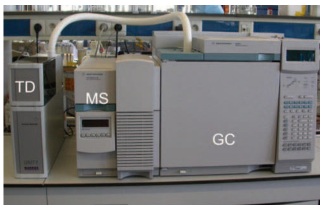
Fig. 49.6 Gas chromatography machinery, including thermal desorber (TD) to release molecules trapped in special collectors, gas chromatograph (GC) for separation of molecules, and mass spectrometer (MS) for identification of molecules.
