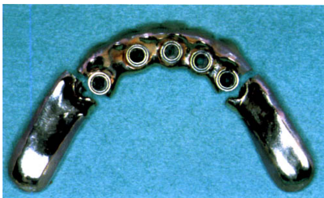
Fig. 10.16 A fractured mandibular fixed prosthesis. Possible causes include mechanical overload, and design and fabrication errors.
