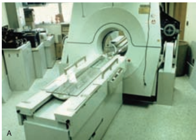
Figure 9.29 (A) Modern head scanners. (B) Note patient table moves into “slicer” at right angle to body axis. Provided by Boston Imaging Associates.
