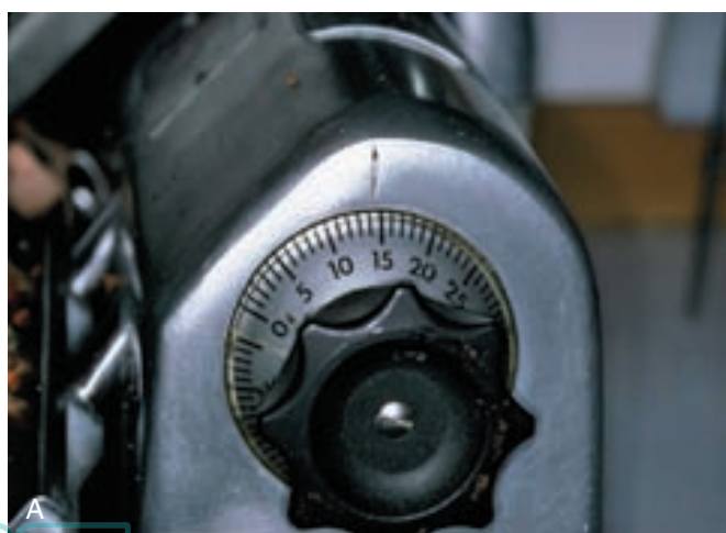
Figure 9.37 (A) Slice thickness selector dial. (B) Variation thickness of slices; thinner slices yield more information.
